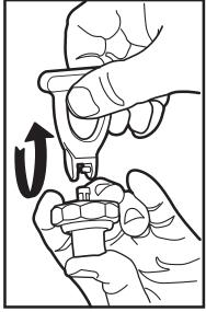
Unlock the shaft from the handle. Compress the spring, pressing down on the bonnet then unhooking the handle.
